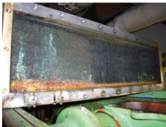
Figure 5: Corrosion de l'intercooler
